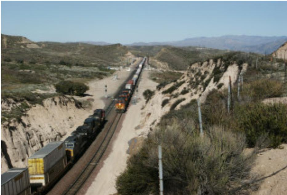
Cajon Pass in California. The train on the left has completed its climb up the mountain and is waiting for the west-bound that is getting ready to descend on the 3% grade. The third track will start in the distance on the left.
