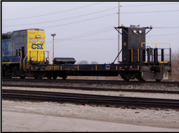
CSX has been using a "Hammerhead" for remote control jobs at Brewer Yard. It allows any MU-capable engine set to be used as remote power, rather than requiring remote-capable locos to be permanently assigned. Image by Doug Nipper.
