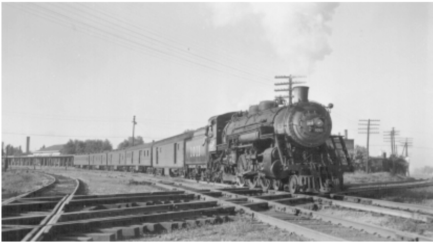
The date is July, 1948 and C&EINo. 1011, a 4-6-2, leads the mail train out of Danville station across the Wabash Railroad at North Yard. This photo is part of Ray Curl's collection acquired by the C&EIHs and Rick Schroeder
