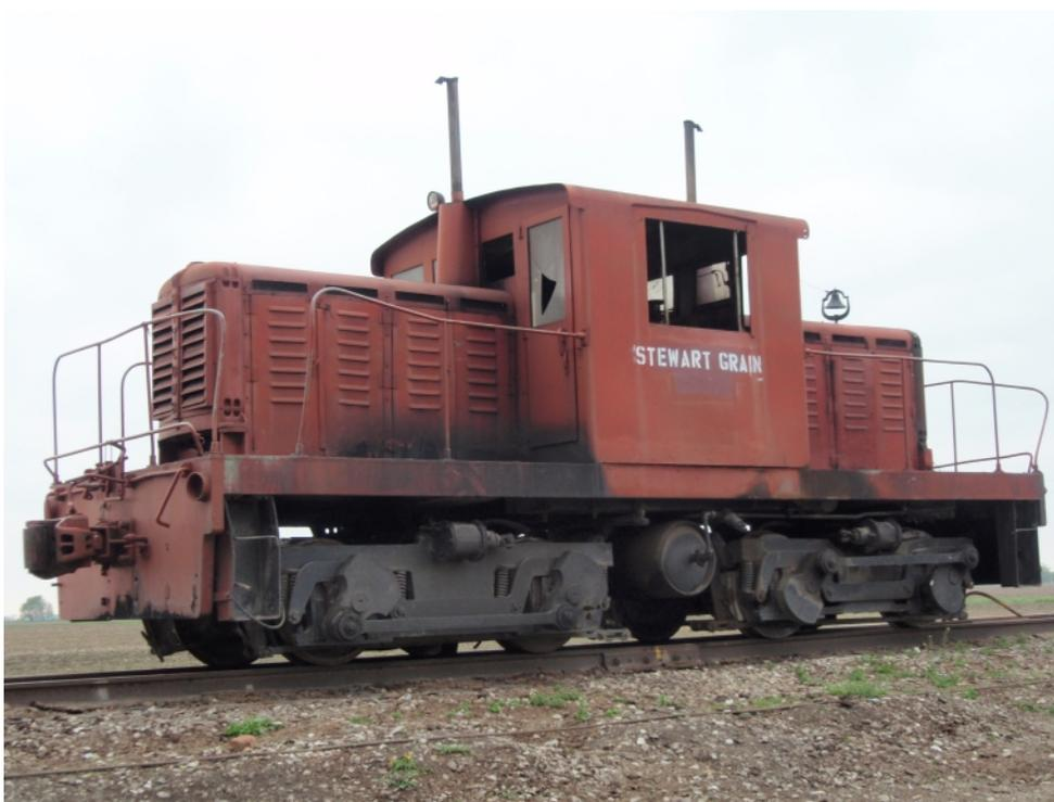
Back in May 2008 the 45-Ton Whitcomb #52 with side rods that used to be at the Rossville, IL elevator was sold to Stewart Grain and moved to Stewart, IN to serve on the "Bee Line" railroad owned by Burt Etchison. Joe Cooke photographed it at Stewart after it was relettered from "Kaufman Grain" to "Stewart Grain".
