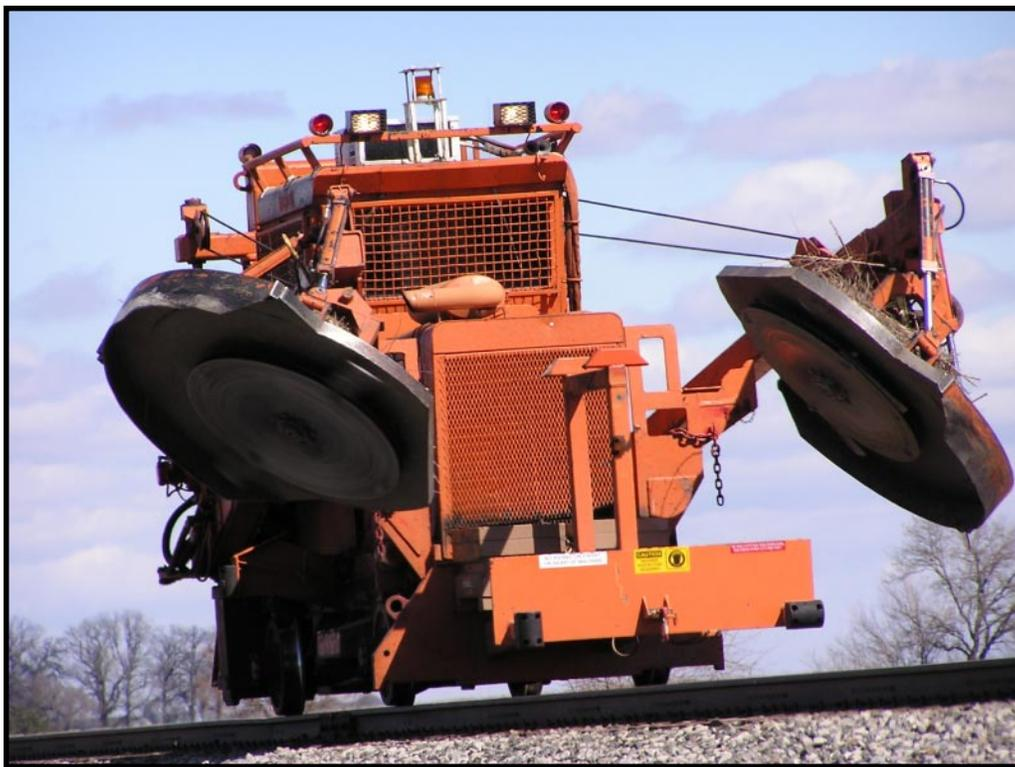
NS brush-cutting crews were out in force late this winter trying to comply with FRA regulations concerning road crossing visibility. Here we see one of the monsters at Marshfield, its booms tucked in to cross a mid-siding road. With the arms extended, the business ends can reach out into virtually any ditch or way up on an embankment. Image by Joe Cooke
